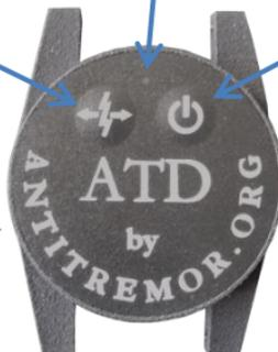
When the ATD is not running, a push on any of the two buttons will start it.
